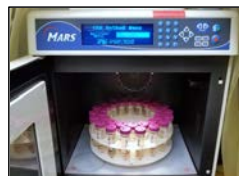
Microwave digestion system: used to enhance the leaching of Pb from the collected soil and dust samples.
